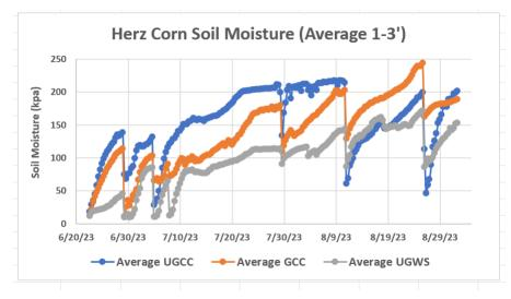
**Figure 4.** Soil moisture depletion (average of 0-36") for June-August 2023 corn in Nuckolls County. All treatments began the season with soil moisture below field capacity in the three-foot soil profile. In fact, there was no moisture below 22" when the soil moisture sensors were installed. The ungrazed cover crop (UGCC) treatment reached 50% depletion (150 kpa) by July 10, grazed cover crop (GCC) treatment by July 25, and ungrazed wheat stubble (UGWS) by August 17.
