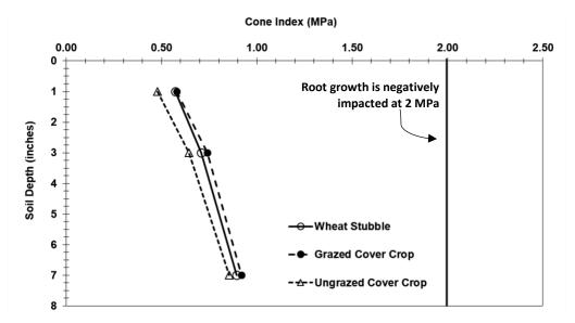
**Figure 2.** Three-year follow-up soil cone index values by treatment taken August 5, 2019. The line on the far right represents where root growth is negatively impacted, because roots are no longer able to easily penetrate through the soil.
