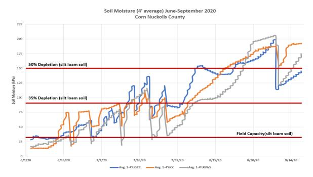
**Figure 3.** Soil moisture depletion for June-September 2020 corn in Nuckolls County. All treatments began the season with soil moisture at or above field capacity. The ungrazed cover crop (UGCC) and grazed cover crop (GCC) treatments reached 50% depletion by mid-August with the ungrazed wheat stubble (UGWS) reaching 50% depletion toward the end of August.
