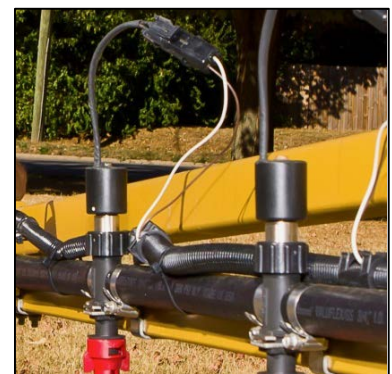
The Capstan Ag PWM nozzle control system may extend flow rates over 6:1 across the range of typical operating pressures.
