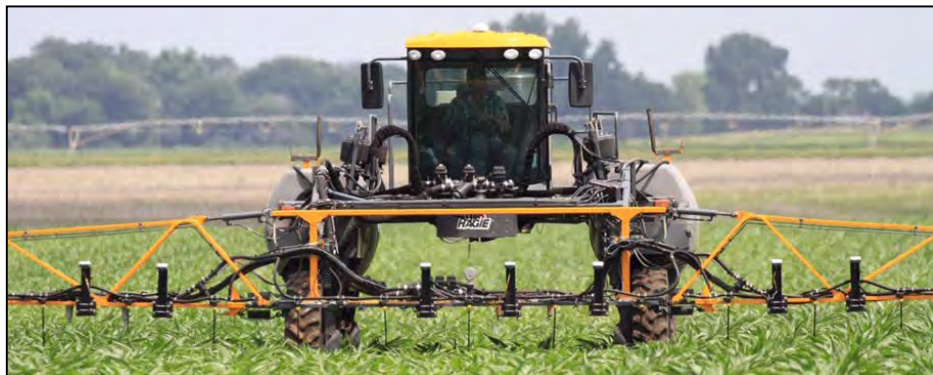
Figure 3: High clearance applicator equipped with OptRx® crop canopy sensors, GPS, and drop nozzles.
