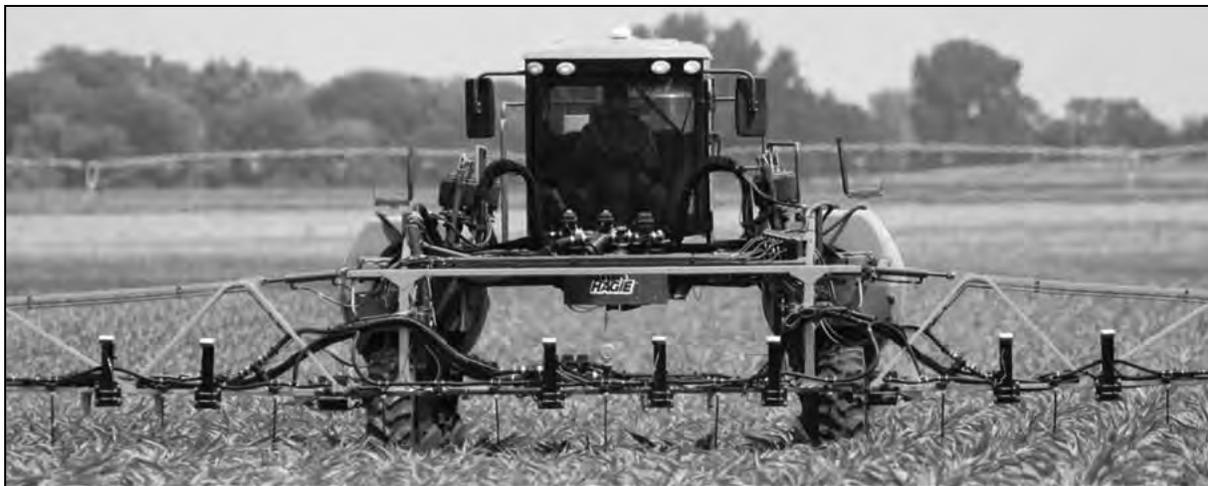
**Figure 3.** High clearance applicator equipped with OptRx<sup>®</sup> crop canopy sensors, GPS, and drop nozzles.
