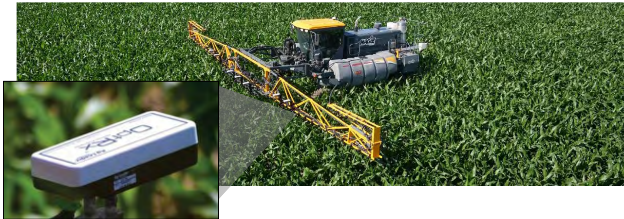
Figure 1. High clearance applicator equipped with OptRx ® crop canopy sensors, GPS, and drop nozzles (above) and active crop canopy sensor positioned over corn canopy (left, inset).
