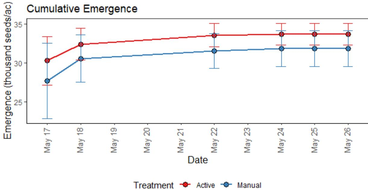
**Figure 1.** Cumulative emergence by date for manual downforce and active hydraulic downforce with the Precision Planting® DeltaForce® system.
