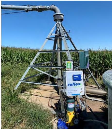
**Figure 3.** Center-pivot system equipped with a variable rate fertilizer injection pump.
