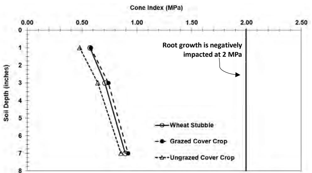
**Figure 2.** Three-year follow up soil cone index values by treatment taken August 5, 2019. The line on the far right represents where root growth is negatively impacted, because roots are no longer able to easily penetrate through the soil.
