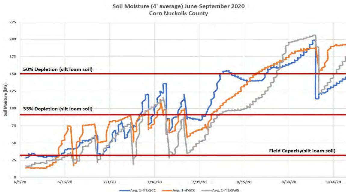
**Figure 3.** Soil moisture depletion for June-September 2020 corn in Nuckolls County. All treatments began the season with soil moisture at or above field capacity. The ungrazed cover crop (UGCC) and grazed cover crop (GCC) treatments reached 50% depletion by mid-August with the ungrazed wheat stubble (UGWS) reaching 50% depletion toward the end of August.
